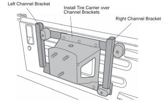
Use Bumpers and pre-existing Fasteners where available to install Channels. Where holes are not available, install Jack Nuts.
