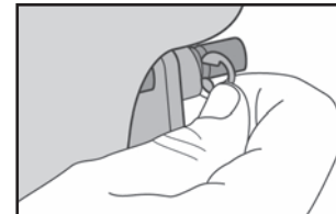
Install Right Front Mounting Bracket on Seat with E-Clip
