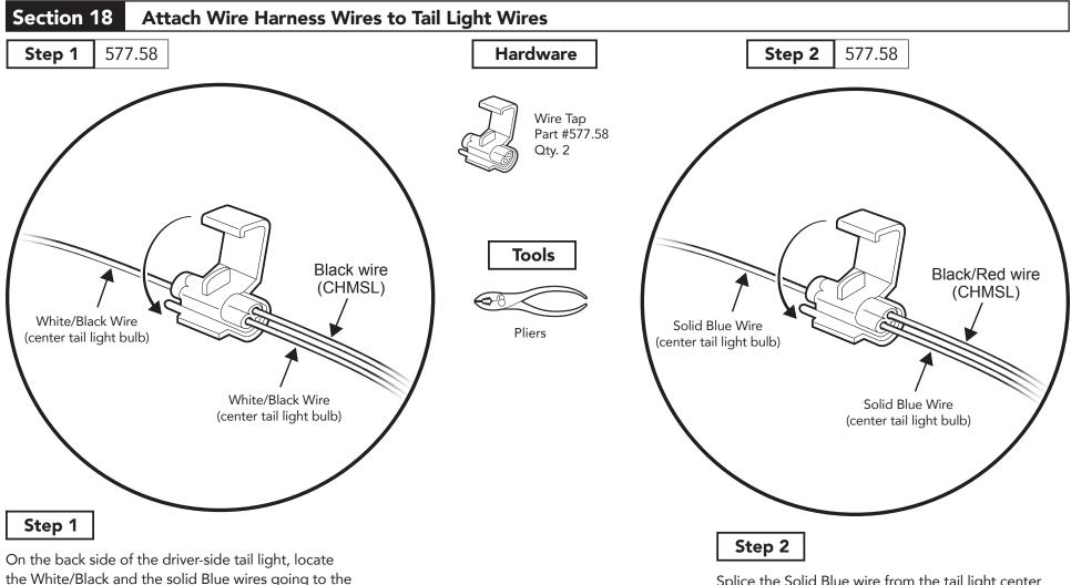
Splice the Solid Blue wire from the tail light center bulb to the Black-Red wire from the CHMSL, using a Wire Tap #577.58 and a pair of pliers.
