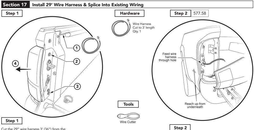
Cut the 29" wire harness 3' (36") from the end with the connector. Feed the cut end underneath the vehicle bed rail cap at location ① and through the slot underneath the edge of the cap. Leave about 5" of the wire harness with the connector inside the vehicle bed.
