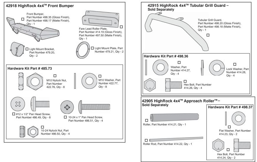
**NOTE** If you intend to install a fare lead roller and/or a winch on your bumper, you will need to install them on the bumper before you install the bumper on the vehicle.
