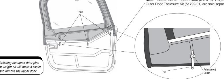
*Note: Lubricating the upper door pins* with a light weight oil will make it easier to install and remove the upper door.
