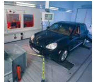
Cold-starting properties of the spark plugs are tested on the two-axis mobile testing stand in BERU's Ludwigsburg Research and Development Centre.
