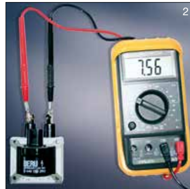
Secondary resistance test
