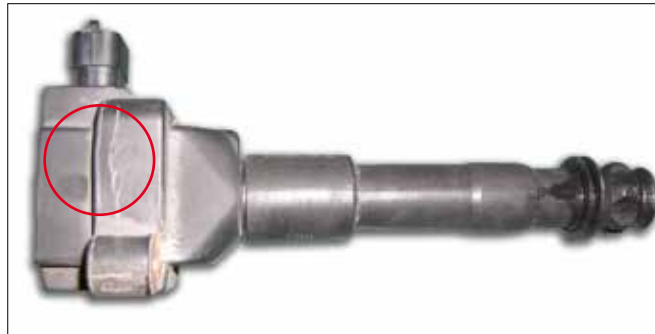
Formation of longitudinal cracks on coil body due to incorrect and excessive tightening torque of 15 Nm instead of the correct 6 Nm.
