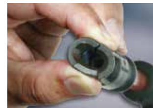
The hairline cracks are clearly visible by pressing the spark plug connector.
