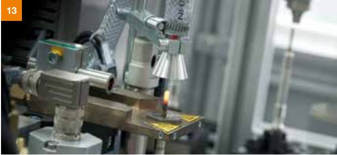
13 100% functional testing of the PSG: The glow test proves that the plug reaches the required temperature in the allotted time.
