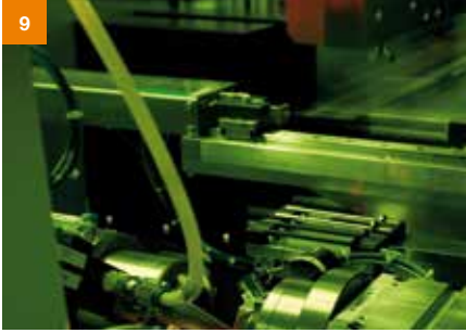
9 In the 6th module the sensor is laser welded onto the extension.
