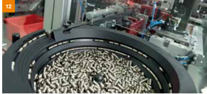
12 To achieve flexible bearing of the heating rod, the glow tube is surrounded by a boot. The figure shows the boot feeding via a conveyor rail.
