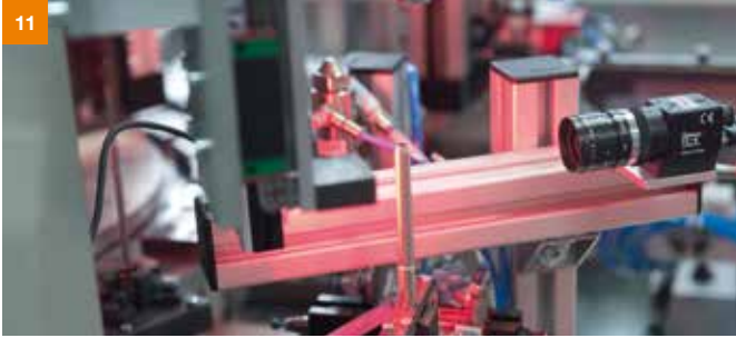
11 Feeding of the glow plug upper part is monitored and documented by a camera.
