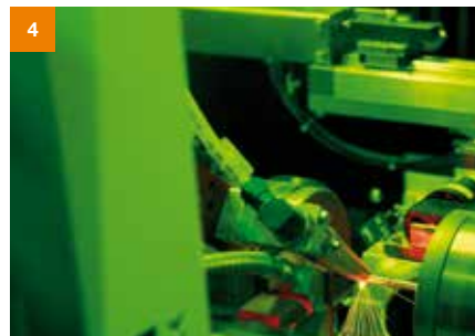
The heating element and extension are laser welded in the 2nd module.
