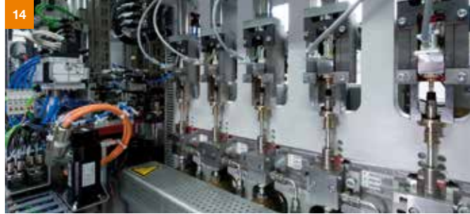
14 Then leak testing is performed.
