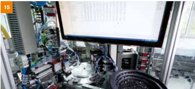
15 This is now followed by geometry testing of the plug: The final dimensions and precise concentricity are documented by a camera system.
