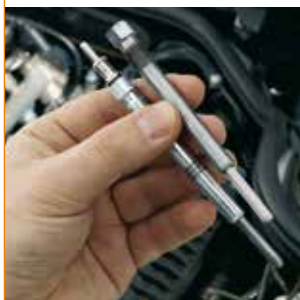
The BERU reamer – (RA003 – 0 890 100 003) loosens coking that might occur after „baking-on„ between glow plug and cylinder head.
