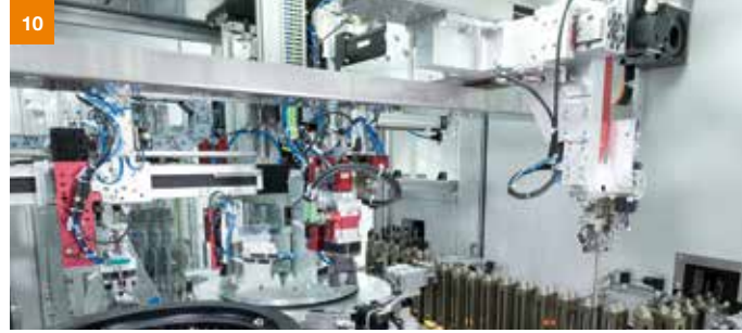
10 In the logistics module, the parts are moved from the first to the second production train, where pre-assembly of the end cap initially takes place.
