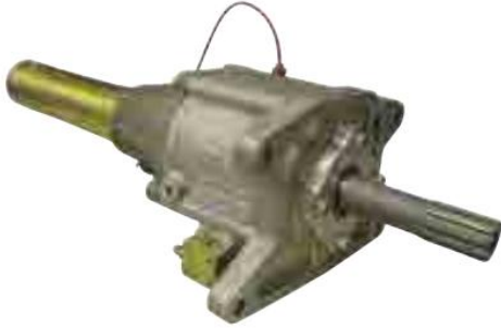
Late Model Transmission 2 nd Generation Muncie Length Tailhousing 3" Longer to fit Muncie Length SG-1400
