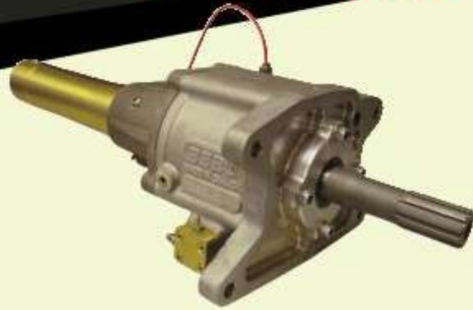
Late Model Transmission 2 nd Generation Muncie Length SG-1400
