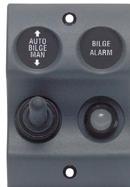
900-BA Bilge alarm and bilge pump control panel includes: 1 on/off/on switch for auto manual control; 1 warning light and alarm for high water level alarm. (Float switch ordered separately - Part # SB1-FS)
