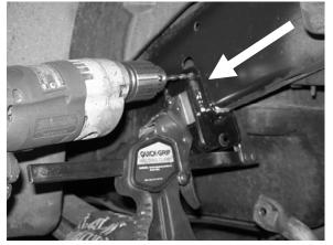
**STEP 1E:** Un–clamp the END LINK BRACKET, removing it from the chassis frame. Using a 3/8" drill bit, clearance the three existing holes in the chassis tube frame.
