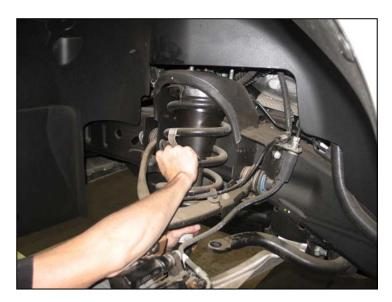
! Coil springs may be under tension. Springs under tension store a great amount of energy. Use caution during the following steps to avoid personal injury and/or damage to vehicle. Be careful not to damage the brake hoses.
