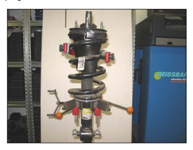
5b. Using an 18mm socket wrench, remove the top mount.
