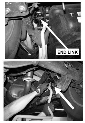
**STEP 3C:** Tighten both hardware to torque specs.
