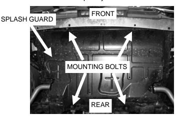
**B.** Using a 10mm wrench, or an air ratchet with a 10mm socket head, remove all four screws.
