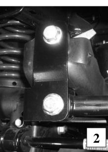
3h) Check all of the hardware and re-torque at intervals for the first 10, 100, and 1000 miles.
