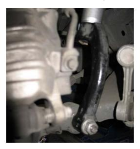
2d. Slide shock yoke off its retaining pin and remove the strut assembly.
