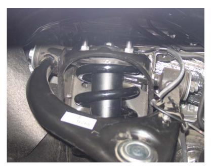
2c. As you did for the top mounts, remove the bottom mounting bolt of the spring/strut assembly.
