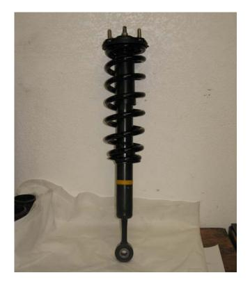
! Coil springs may be under tension. Springs under tension store a great amount of energy. Use caution during the following steps to avoid personal injury and/or damage to vehicle. Be careful not to damage the brake hoses.
