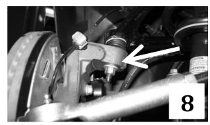
5b. Re-install the sway bar end links to 18ft-lbs.
