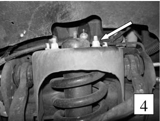
2e) Remove the top three mount bolts of the front spring/strut assembly. (**photo 4**) Slide the spring and shock assembly down and out of the front suspension. For ease of reinstallation, mark the outboard side of the spring and upper shock mount with a paint pen.
