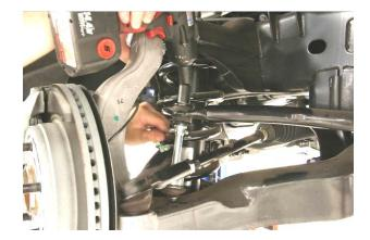
C. Loosen the two lower shock bolts holding the shock bar pin to the lower control arm with a 13mm socket.
