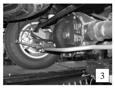
lower end-link to the ASB using the supplied bolts, washers and lock nut hardware. The ASB should be on the inside of the end link assembly and the bolt should be fed from the inside. Tighten the hardware to 74 ft lb using a socket and wrench.
