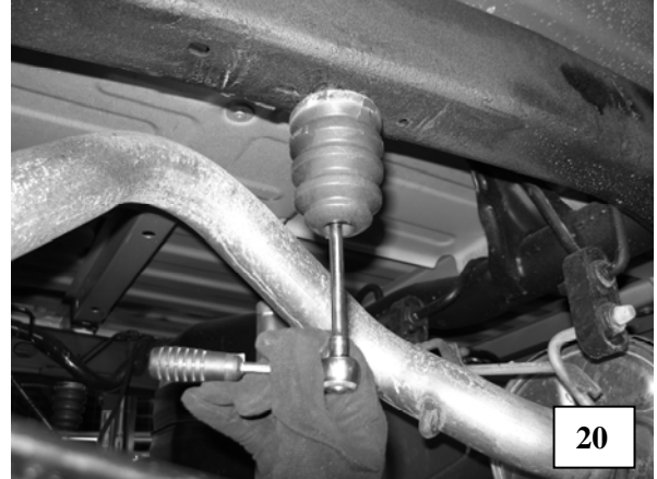
DRILL A PILOT HOLE FOR THE SELF THREADING BOLT
