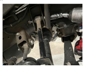
11. Remove the outer bolt and remove the upper control arm from the vehicle.
