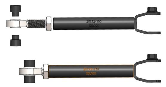
13. Preset the length of the adjustable control arm and set by tightening the jam nut to prevent adjustment from moving during the installation process. To achieve lowering between 3" to 4",set the distance from center to center at 320mm (12.59").
