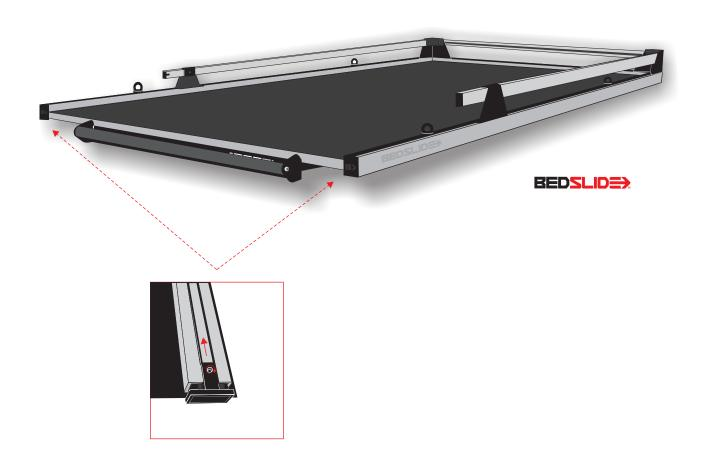
**Supplied Hardware**: (4) 5/16 riv nuts, (1) riv nut tool, (4) 5/16 x 2" hex head bolts, (4) 5/16 split lock washers, (4) 3/8 flat washers
