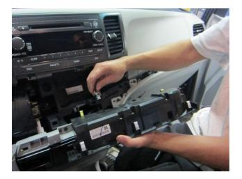
7. Remove the (4) 10mm screws, (2 each side that secure the radio head unit) use a 1/4 drive socket, not power tools to remove. Be careful not to let the 2 screws toward the back fall down inside the dash area when removing.
