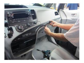
2. Squeeze the plug on the wire harness to release it from the trim panel.
