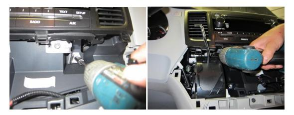
8. Carefully pull the radio head unit out towards you to release it from the dash after removing the (4) 10mm screws.
