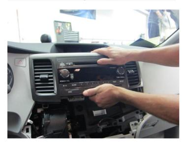
9. Remove wire harness from back of factory radio by carefully squeezing the clips until they release, DO NOT PULL ON THE WIRES! Remove antenna, etc., and take head unit to work table to Remove and replace the A/C vents and radio side brackets.
