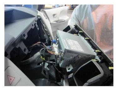
10. Disconnect 5-pin (PKB, VSS) and 1-pin (GPS) connectors from the screen.
