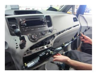
3. Unscrew the shift handle counter clockwise to remove. Use your fingers to carefully pry up the shifter cover starting from the bottom.
