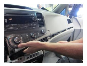
6. Unclip the harness from the back of the climate control, and set aside. Be careful when handling the dash trim parts so they don't get scratched or damaged.
