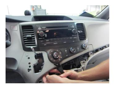
4. Lift the cover over the handle, and let dangle on the left side of the dash, out of the way, or you can disconnect the plug on the back and set aside.
