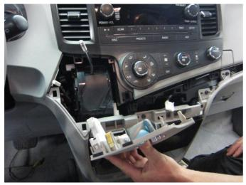
5. Using your fingers, pull straight out on the climate control and carefully wiggle the unit, pulling towards you until the clips release.
