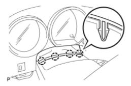
(a) Detach the 4 claws and remove the instrument panel finish panel retainer.
