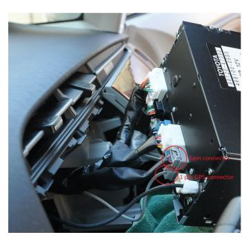
Remove the 6pin gray connector and the 1pin GPS connector circled above in red and daisy-chain it with the TVK-10 connectors. (OEM connector to TVK-10, TVK-10 to NAV unit)
