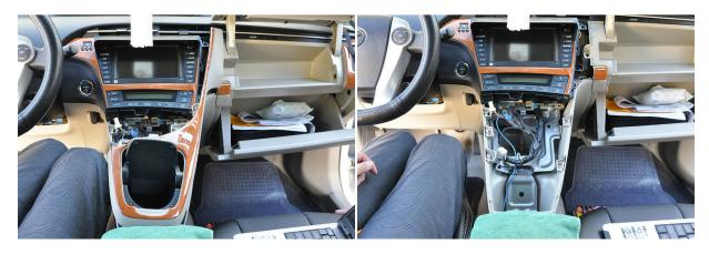
Open the cup holder and loosen the clips around the cup holder. Then, work your way up and loosen the side piece. Be careful not to pull too hard or bend the long piece.
