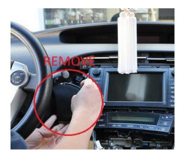
Remove the panel with the "START" button. Also disconnect the connector behind this piece and place it in a safe location.
