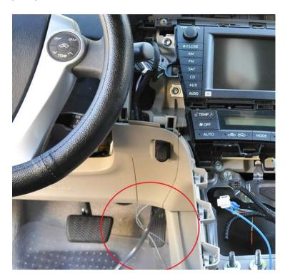
Route the TVK-10 line to behind the center console. Do this before you place the navigation unit back to the factory mounts. There is space behind the navigation unit where the line can be routed.
