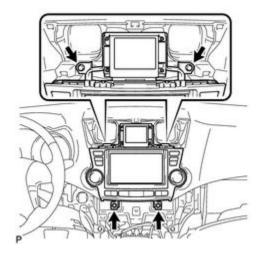
(b) Pull the navigation receiver assembly with bracket toward the rear of the vehicle and disengage the 4 clips.
