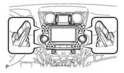
(c) Disconnect each connector and remove the navigation receiver assembly with bracket.
