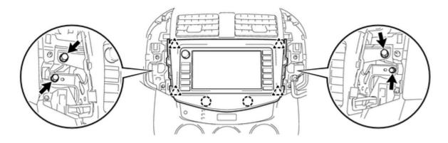
(2) Pull the navigation receiver to detach the 2 claws and 4 clips on the backside of the navigation receiver.
