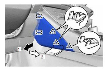
(b) Pull the instrument panel finish panel end LH in the direction indicated by the arrow (2) shown in the illustration to disengage the 2 guides and remove the instrument panel finish panel end LH.
