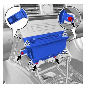
(b) Pull the radio receiver assembly with bracket toward the rear of the vehicle and disengage the 4 clips.
