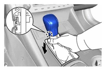
(b) Turn the shift lever knob sub-assembly counterclockwise and remove it.
