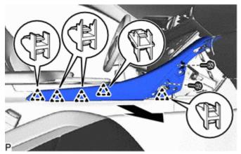
(b) Disengage the 5 clips to remove the front panel garnish RH.
