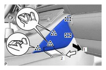
(b) Pull the instrument panel finish panel end RH in the direction indicated by the arrow (2) shown in the illustration to disengage the 2 guides and remove the instrument panel finish panel end RH.
