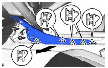
(b) Disengage the 5 clips to remove the front panel garnish LH.
