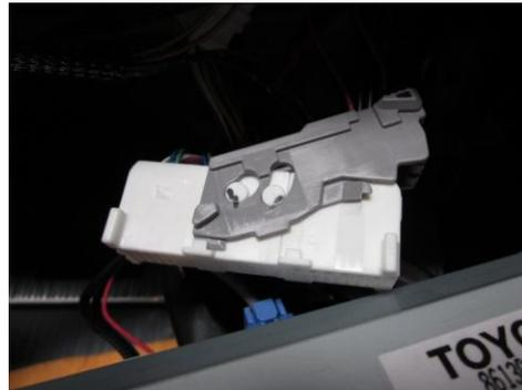
(h) Once the main connector is in one piece with the gray bracket, insert it back to behind the oem head unit.
