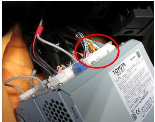
(b) Take a flat head screw driver to release the clip on the right side of the connector. Then pull the connector out.
