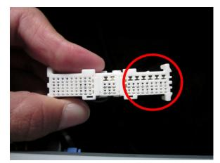
(e) Connect the male side of the NDS6223EP connector to the female connector which was disconnected from the previous step. Make sure the connection is secure and that none of the pins are exposed on the side.
