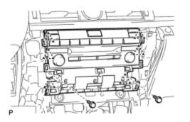
HINT: Grab a towel and rest the radio between the towel and center console to avoid scratching interior pieces.
