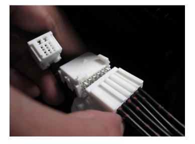
(f) Take the female side of the NDS6223EP connector and link it back to the main connector, then mount the gray bracket back to the main connector.
