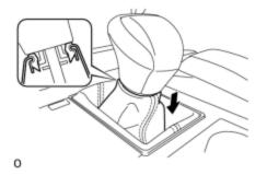
(b) Twist the shift lever knob sub-assembly in the direction indicated by the arrow and remove it.
