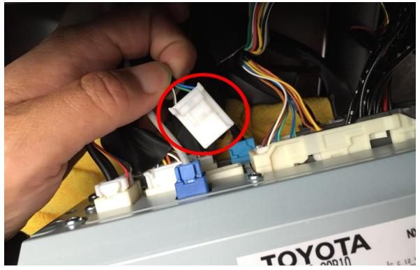
• Connect the matching connector on the NDS6223EP to the factory steering wheel control connector what you just disconnected from the head unit.
