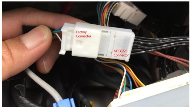
• Connect the other side of the NDS6223EP connector to the factory head unit.
