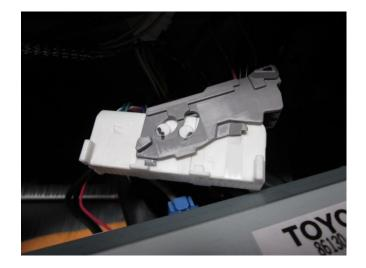
(g) Once the main connector is in one piece with the gray bracket, insert it back to behind the oem head unit.
