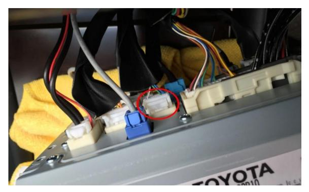
• Disconnect the steering wheel control connector.
