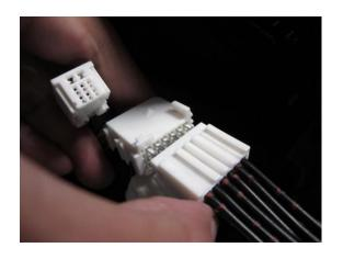
Using the supplied urethane insulation tape, tear off a size to cover the 2, 24 pin connectors that are mated to each other as shown on the right.
