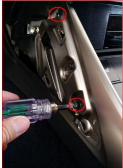
Remove the side molding by using a panel removal tool. Start to pry out from the bottom right corner as shown on the right picture.
