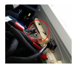
Take a flat head screw driver to release the clip on the right side of the connector. Then pull the connector out.
