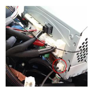
Locate the matching connector behind the factory head unit as shown on the photo.
