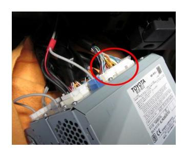
(b) Take a flat head screw driver to release the clip on the right side of the connector. Then pull the connector out.
