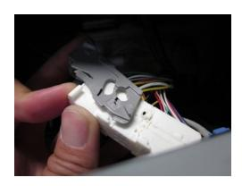
(d) After the gray bracket is removed, the connector should look like this. The right side of the connector is what you need to disconnect from the main connector.
