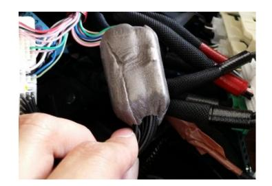
(g) Take the female side of the NDS6223EP connector and link it back to the main connector, then mount the gray bracket back to the main connector.
