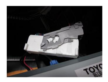
(h) Once the main connector is in one piece with the gray bracket, insert it back to behind the oem head unit.
