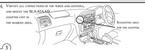
Check to see all connections are secure, all items are firmly in place. Check head unit functions and all vehicle controls before engaging electrical power or any test drive.
