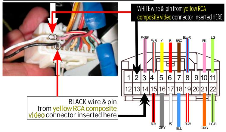
Please verify PIN WIRE COLORS on the MALE side of the M6 modular connector attached to back of the Multi-Display chassis.
