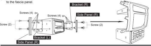
4. Attach the L&R OEM brackets to climate control, display and brackets (2 OEM Screws x 2, supplied nuts x 2) Screw (1) .... Screw (1) Nut (2) -- Screw (1) Screw (1) OEM Bracket (L OEM Bracket (R)
