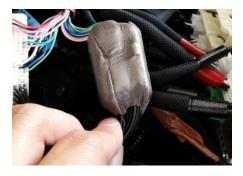
Take the female side of the NDS6223EP connector and link it back to the main connector, then mount the gray bracket back to the main connector.
