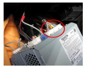
Take a flat head screw driver to release the clip on the right side of the connector. Then pull the connector out.
