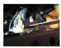
Carefully remove the gray bracket, which is being used to keep the three connectors together.
