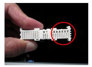
Connect the male side of the NDS6223EP connector to the female connector which was disconnected from the previous step. Make sure the connection is secure and that none of the pins are exposed on the side.
