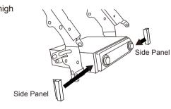
2.4 Re-attach the side brackets to the EMV Audio Assembly taking care to align the locating points on both sides and insert the newly installed aftermarket head unit into the
