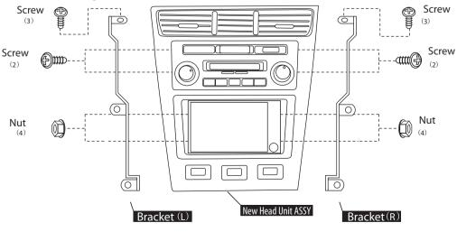
4. Audio, airconditioner controller unit ASSY is attached to the vehicle.
