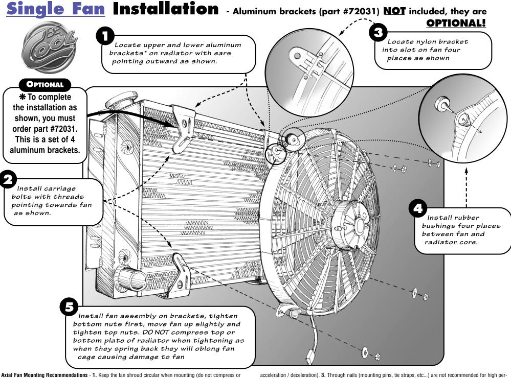
**Axial Fan Mounting Recommendations** - **1.** Keep the fan shroud circular when mounting (do not compress or oblong the shroud). An oblong shroud will cause blade contact within the shroud possibly breaking the fan blades. **2.** When mounting fans larger than 11 inches in diameter, a spacing distance of 1/4 (min) to 1/2 (max) an inch between the base of the shroud and the radiator surface is required. (This protects against blade flex due to vehicle
