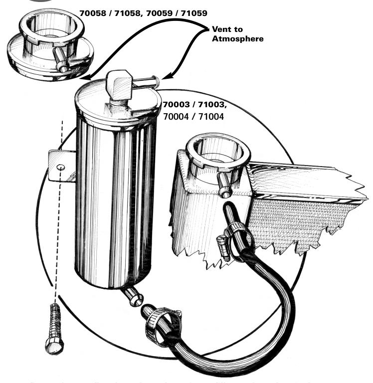
Route the overflow hose from the <u>radiator</u> filler neck to the nipple on the bottom of the recovery tanks.
