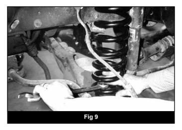
23. Install the appropriate BDS shocks at this time. Tighten upper stem till bushings start to swell. Lower bolt torque to 40 ft.lbs.
