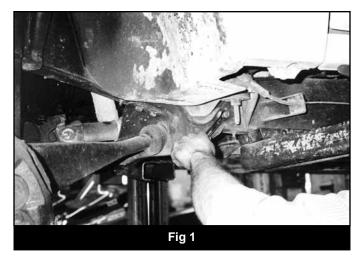
6. Install BDS radius arm drop brackets. It may be necessary to remove the bracket around the fuel system in order to gain space for access to the bolt holes. Install the BDS drop brackets with 6 - 7/16 x 1-1/4. Re-use two OE bolts per bracket with the OE dual nut bracket. When brackets are in place, torque the fasteners to 60 ft.lbs. (Fig. 2)
