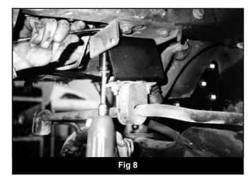
21. Remove the OE pitman arm using an appropriate puller. Install new BDS pitman arm and torque to 170 ft.lbs. Attach steering linkage to the pitman arm and torque to 45 ft.lbs. Be sure to install new cotter key.
