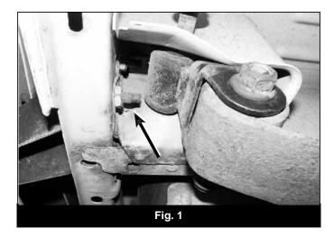
7. Install the new shackles in the OE locations with the original hardware. Leave the spring and shackle bolts loose at this time. The grease fittings should be toward the front of the vehicle (Fig. 2).
