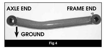
26. Install the straight grease zerk into the axle end of the lower control arm. (Fig 5)
