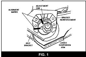
Remove the lower suspension arm nut, cam, and cam bolts from the axle as shown in figure 2.
