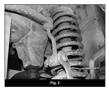
7. Disconnect the sway bar links from the axle. Remove the nut and the sway bar link from the bolt (Fig 2). Some early models will require a T55 torx socket to hold the bolt from rotating. Later models used a bolt with a serrated neck that is pressed into the bracket so it will not rotate. Save axle mount hardware.
