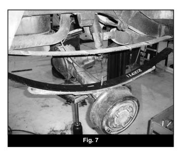
41. Using the C-clamps on each side of the center pin hole, compress the leafs together while aligning the new center pin through all of leaf center pin holes (from the bottom up). With the pack completely compressed together with the
