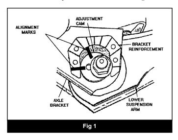
3. Remove the lower control arm nut, cam, and cam bolts from the axle. (Fig 2)
