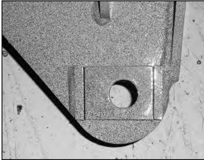
FIGURE 22 - 4" OFFSET TOWARDS DRIVER'S SIDE
